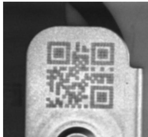
Figure 4-8: Image captured with coaxial lighting
