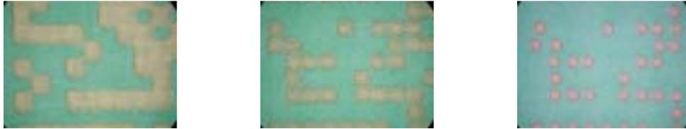
Photo 2-6: Example of cell marking pattern (glass epoxy PCB)
