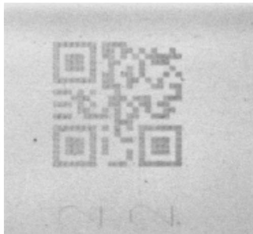
Figure 4-9: Transmitted lighting Figure 4-10: Image captured with transmitted lighting
